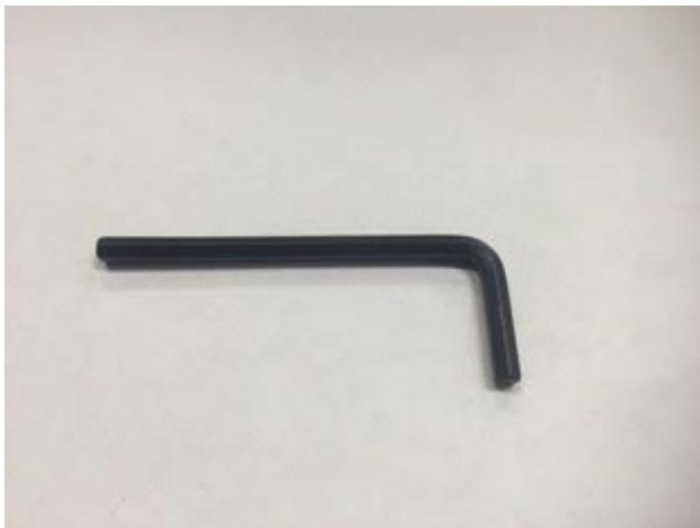
Attach the seat post by placing it into the seat tube, then tighten the seat clamp with a 5mm allen wrench. You can adjust your seat height by loosening this bolt and positioning your seat to a comfortable height.
